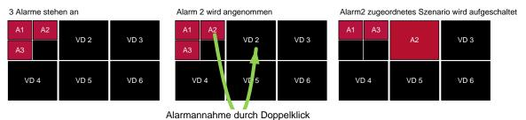
Figure 3-62: Example of an alarm acceptance
