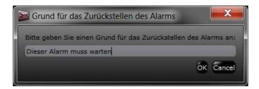
Figure 3-65: Manual entry of the alarm reason when it is returned
